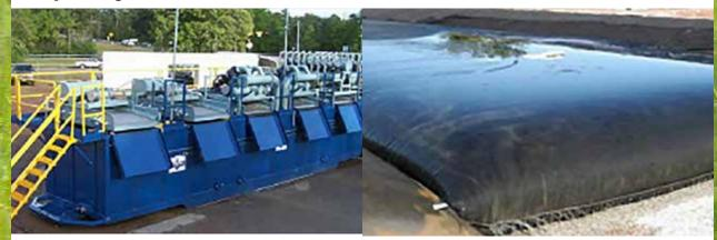
LEFT: Lyngbya is mechanically separated from other suspended material. RIGHT: The remaining liquids are filtered through Geotube bags where a patented polymer mixture is added to facilitate removal of nearly 100% of the phosphorus and about 50% of the nitrogen from the water. Clean water escapes through tiny mesh holes and is collected and returned to the river.
